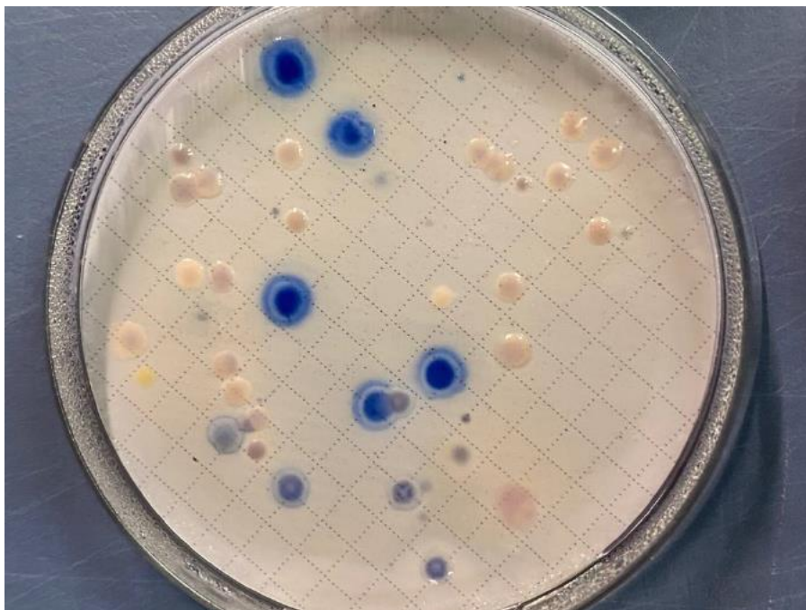
Figure A1. Picture of a fecal coliform membrane filtration growth plate provided by Hillary Eichler from Spectra Laboratories, Tacoma, WA. Blue colonies are fecal coliform, yellow/purple colonies are confluent growth.
