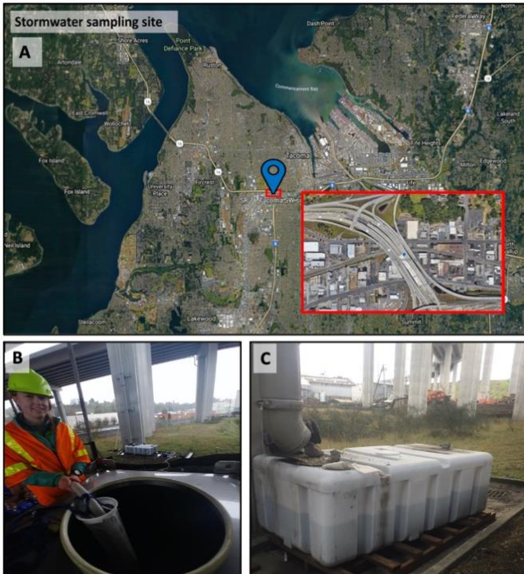
Figure 2. A) Stormwater runoff sampling site location in Tacoma, WA off the junction of I-5 and SR-16. B) Pumping stormwater from the HPDE collection tank into a stainless-steel transfer tank. C) The collection tank collecting water from the highway runoff downspout.
