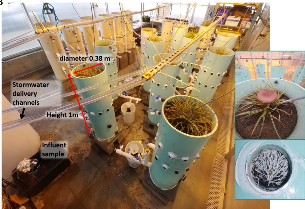
Figure 3. A) Bioretention column experimental design, and B) picture of experimental setup in greenhouse at WSU-Puyallup.
