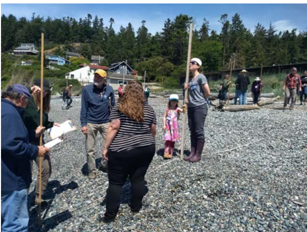
Volunteers learning the "Two-stick Method" for measuring beach profile at Rosario Beach. Photo Credit: Jason Morgan
